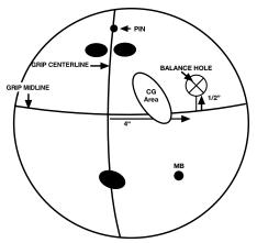
This is the **recommended** layout for most players, with or without a positive axis point. Use mirror image for left handed drilling.
